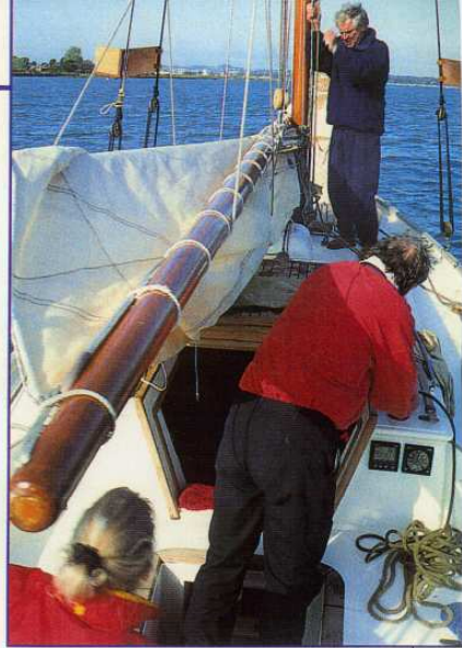
Lazy jacks keep the gaff under control when hoisting the mainsail.
